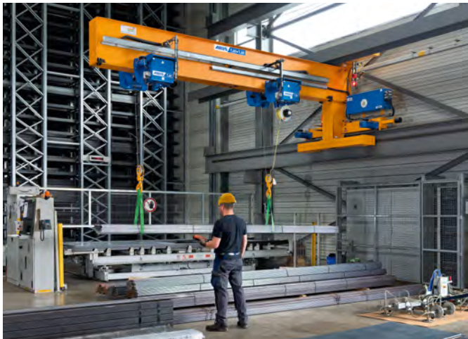
With two hoists in tandem operation, an ABUS EWL single girder wall travelling crane can also be used for the precise positioning of long loads.
