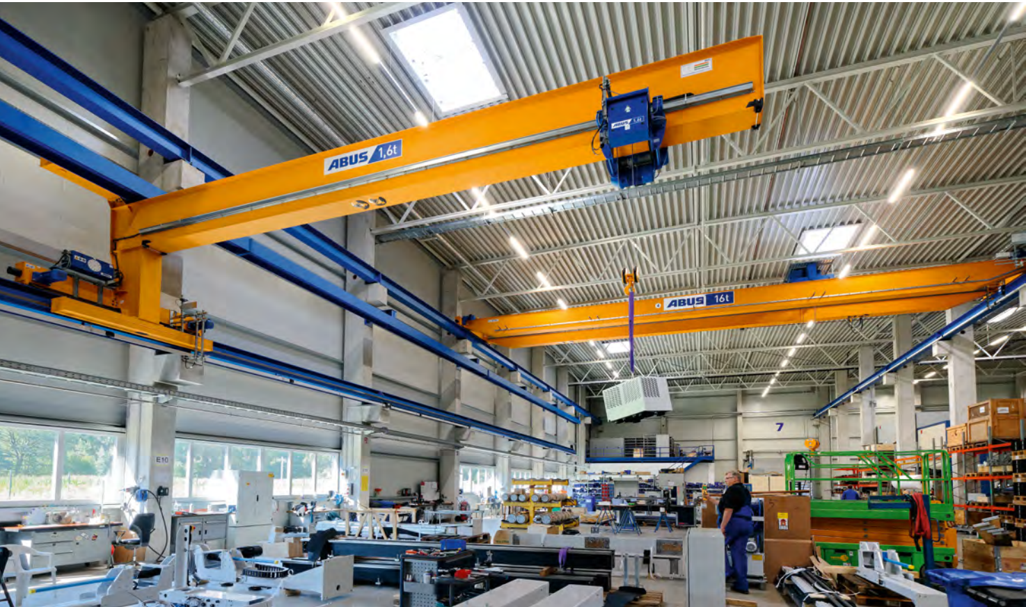
EWL single girder wall travelling crane with electric wire rope hoist
