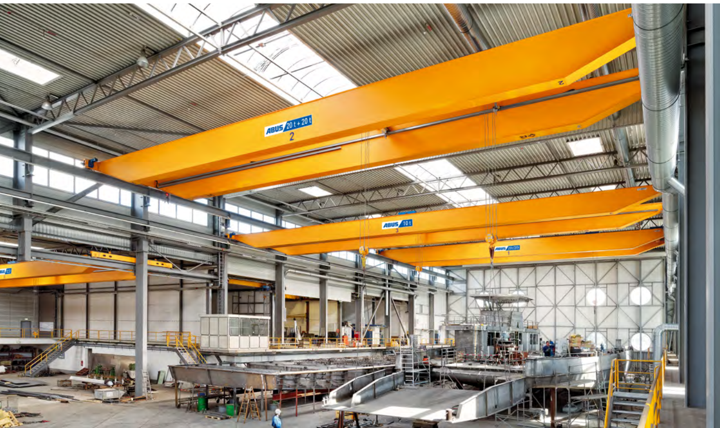
Double girder overhead travelling cranes with welded box girder and standard main girder connection version 1
