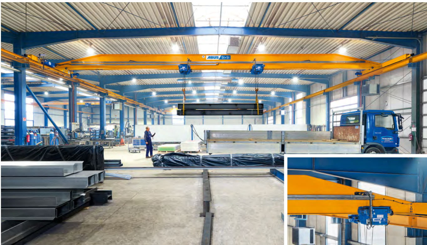
Single girder overhead travelling crane with welded box girder and standard main girder connection version 3. The ideal solution for newly built facilities: the ABUS ELK single girder overhead travelling crane with main girder chamfer adapted to suit the roof haunch. This allows for optimal use of the available height within the facility (can also be achieved with single girder overhead travelling crane ELV with rolled section girder)
