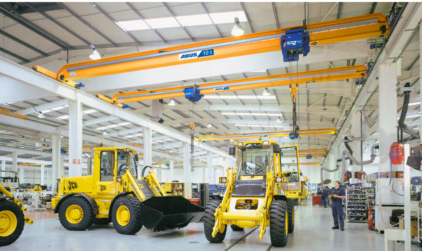
Single girder overhead travelling crane with rolled section girder and standard main girder connection version 3
