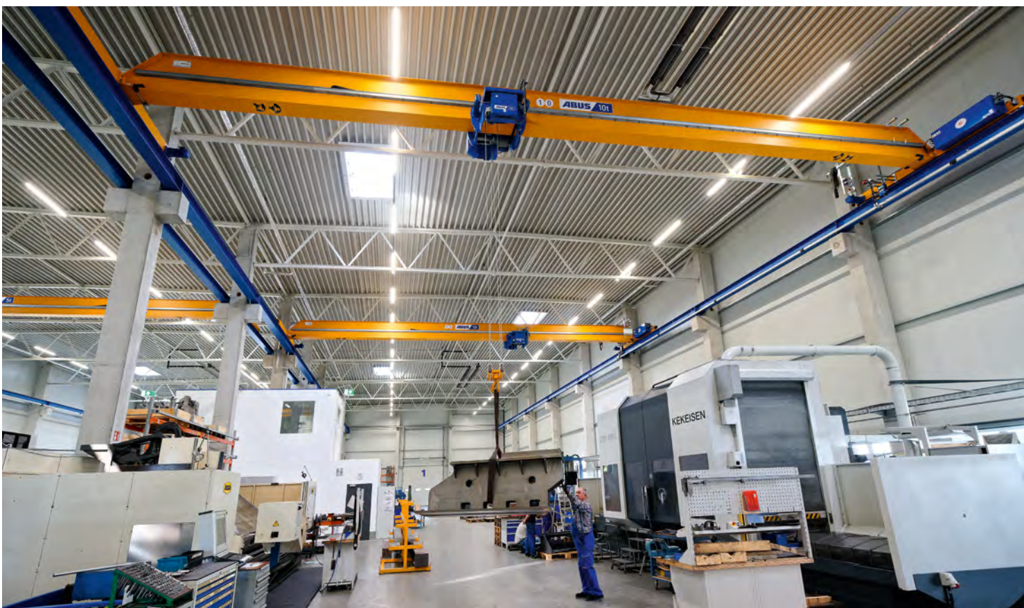
Single girder overhead travelling crane with welded box girder and standard main girder connection version 3
