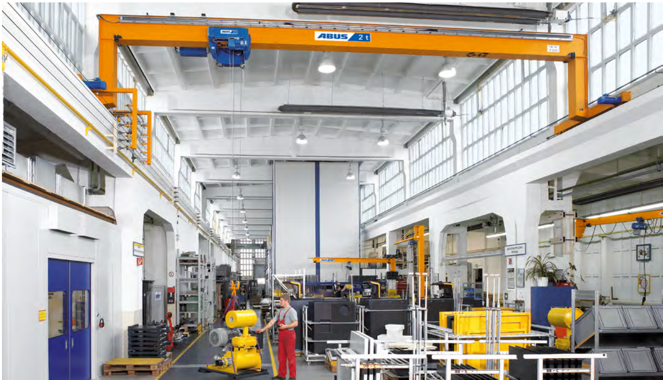
Single girder overhead travelling crane ELK with welded box girder and stooped up main girder connection version 5. In specific architectural applications with structural constraints, stooped-up crane bridges offer an ideal solution (can also be achieved with the single girder overhead travelling crane ELV with rolled section girder)
