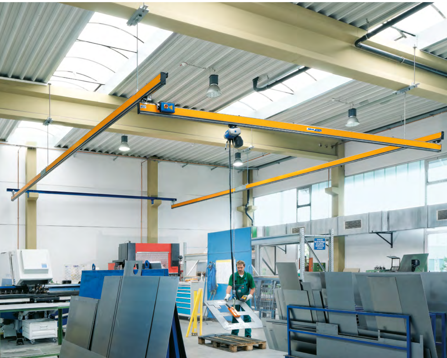
Fitted to a reinforced concrete support beam using an embracing bracket
