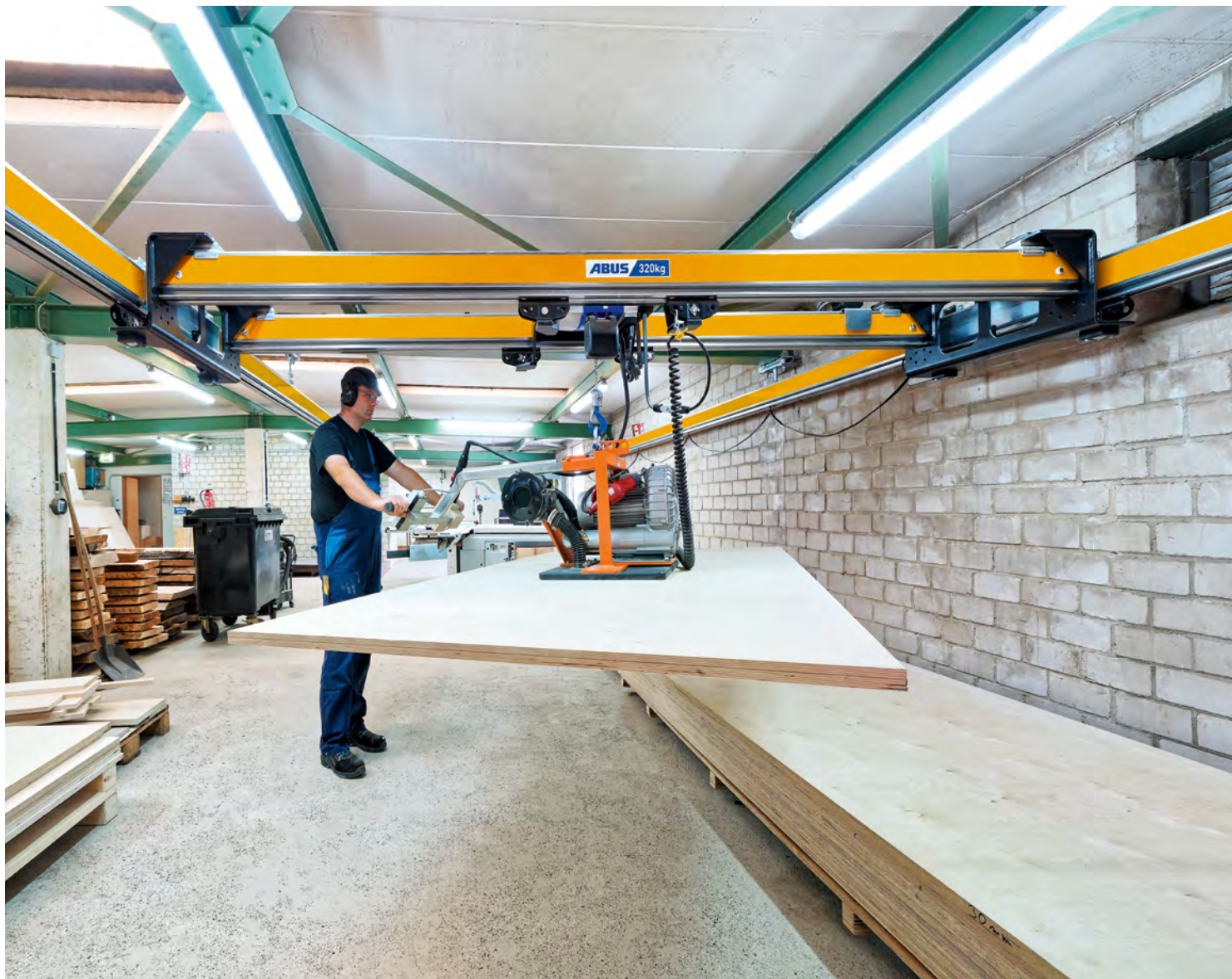
Fitted to rolled section I-beam using clamps and including preparation for vacuum hoist unit
