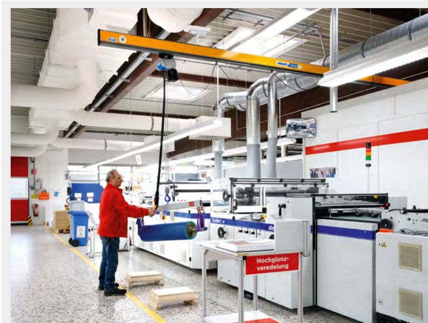
ABUS double rail system For linear point-to-point coverage Load capacity: up to 2 t
